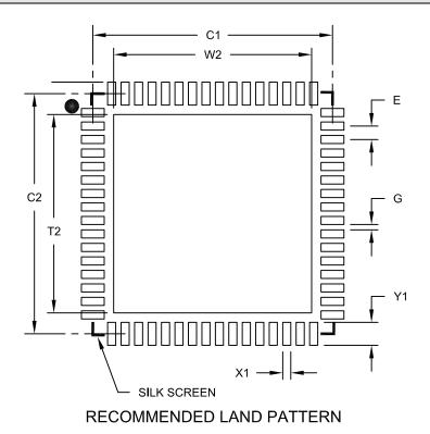
Units **MILLIMETERS** MAX **Dimension Limits** MIN MOM Contact Pitch Е 0.50 BSC Optional Center Pad Width W2 7.35 7.35 Optional Center Pad Length T2 8.90 Contact Pad Spacing C1 Contact Pad Spacing C2 8.90 Contact Pad Width (X64) 0.30 X1 Contact Pad Length (X64) Y1 0.85 Distance Between Pads G 0.20
