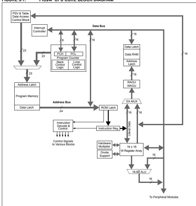
FIGURE 3-1: PIC24F CPU CORE BLOCK DIAGRAM
