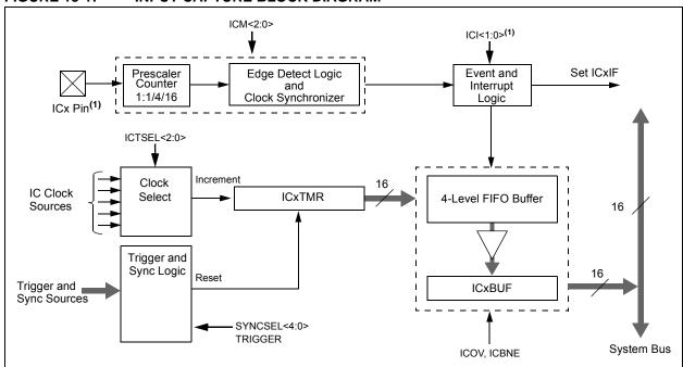
Note 1: The ICx inputs must be assigned to an available RPn pin before use. Please see Section 10.4 "Peripheral Pin Select" for more information.
