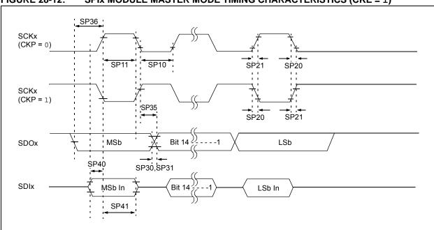
FIGURE 28-12: SPIX MODULE MASTER MODE TIMING CHARACTERISTICS (CKE = 1)
