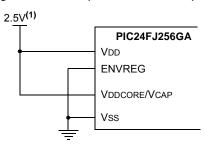
Note 1: These are typical operating voltages. Refer to Section 28.1 "DC Characteristics" for the full operating ranges of VDD and VDDCORE.
