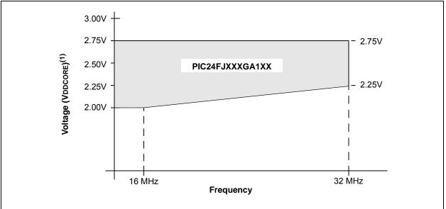
For frequencies between 16 MHz and 32 MHz, FMAX = (64 MHz/V) \* (VDDCORE - 2V) + 16 MHz.
