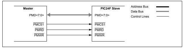
FIGURE 18-3: ADDRESSABLE PARALLEL SLAVE PORT EXAMPLE
