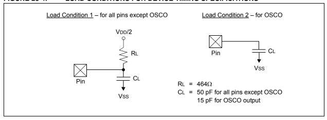
TABLE 28-12: CAPACITIVE LOADING REQUIREMENTS ON OUTPUT PINS
