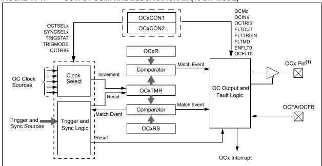
Note 1: The OCx outputs must be assigned to an available RPn pin before use. Please see Section 10.4 "Peripheral Pin Select" for more information.
